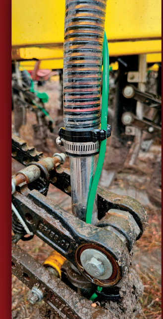
Then open the NITROCLIP to put over the hose. Try not to move the clip after it has gripped the hose to let the grippers work.
